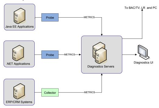
The diagram shows one Diagnostics Server in Commander mode connected to a one or more Diagnostics Servers in Mediator mode. Each Diagnostics Server in Mediator mode is connected to a number of probes or collectors. The Diagnostics probes and the Diagnostics collector capture events from the monitored applications.
