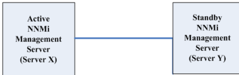
Figure 2 Using Self-Signed Certificates with Application Failover
