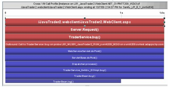
The red nodes in the profile are the processing that took place on the origination system, and the blue nodes are the processing that took place on the child system, **ovrntt209**.
