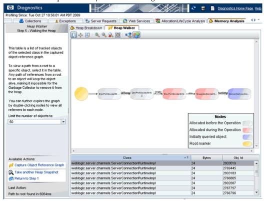
An example of an Object Reference Diagram is shown below:
