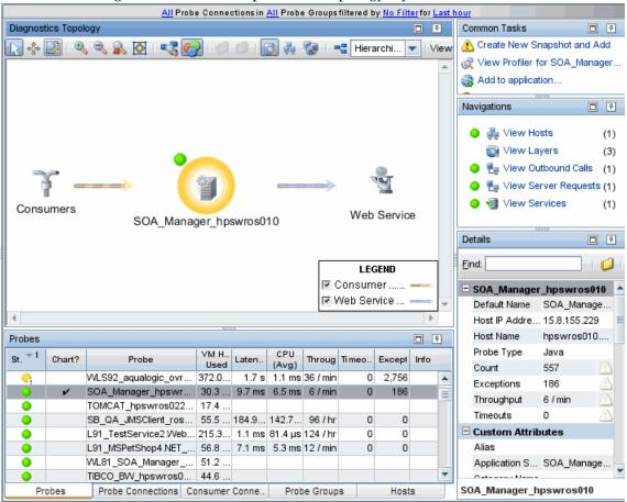
The topology diagram includes a toolbar with controls that allow you to pan, zoom, and alter the way the diagram is drawn by grouping entities, changing diagram type, or changing connection (link) information.
