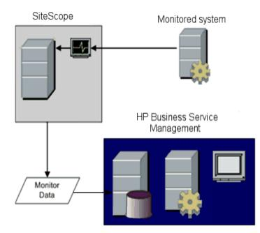
BSM includes a System Availability Management (SAM) Administration page. This function allows you to manage SiteScope monitor configurations for one or more SiteScope servers through a central console. This level of SiteScope integration is separate from the integration of SiteScope monitor data with BSM.
