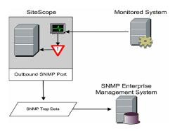
The following diagram illustrates the SNMP Trap Alert.
