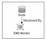
The Node CI has a monitored by relationship with the EMS Monitor CI. The EMS Monitor CI passes status onto the Node CI.
