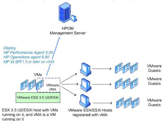
The illustration shows that the HP Performance Agent, HP Operations agent, and the VI SPI are deployed on a vMA, which is a virtual machine hosted on a VMware ESX/ESXi host. It is used to perform most of the tasks performed in the ESX/ESXi service console. vMA is a standard used to run scripts or agents that manage VMware ESX/ESXi hosts and guests.
