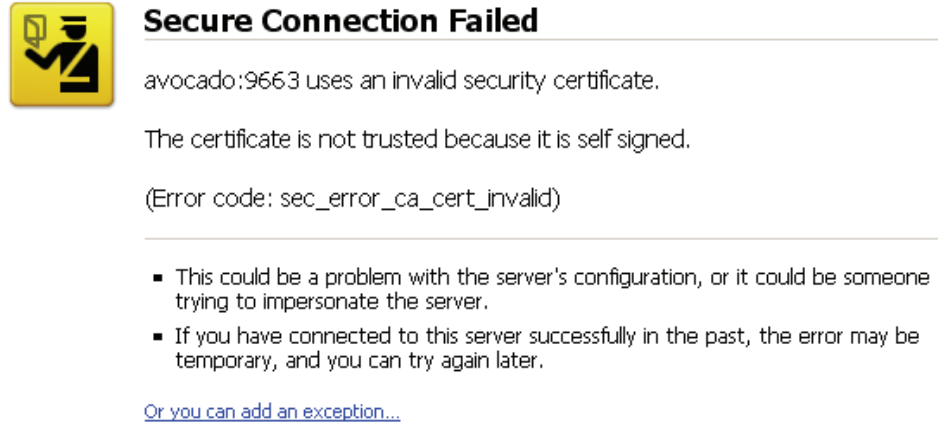
Figure 13 Self Sign Warning
