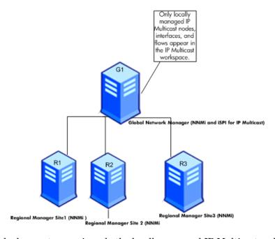
In this deployment scenario, only the locally managed IP Multicast nodes, interfaces, and flows are available in the IP Multicast inventory (G1).
