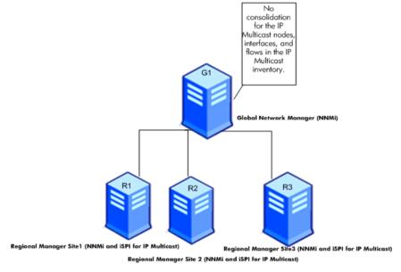
In this deployment scenario, all the Regional Managers (R1, R2, and R3) discover the IP Multicast nodes, interfaces, and flows. The iSPI for IP Multicast is not available on G1 so there is no communication established between G1 and regional managers for the iSPI for IP Multicast. Thus, the Multicast nodes, interfaces, and flows from the Regional Managers are not available in the G1 inventory. In addition, no aggregated IP Multicast reports are available in the IP Multicast (GNM) inventory.
