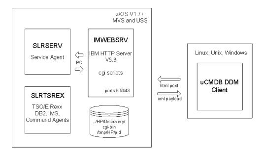
The IBM HTTP Server needs to be up and running in order for SLRSERV to work correctly. See Chapters 4 and 6 of the *HTTP Server Planning, Installing, and Using* manual.
