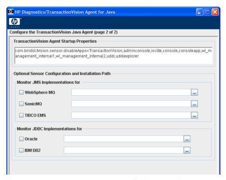
The Transaction Agent Startup Properties field contains directives as to the operation and instrumentation of the Agent. Typically you should accept the default unless instructed otherwise by HP Customer Support. The properties are separated by semicolons.
