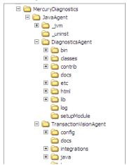
The default location of <java\_agent\_install\_dir> is C:\MercuryDiagnostics\JavaAgent\ on Windows and /opt/MercuryDiagnostics/JavaAgent/ on UNIX.
