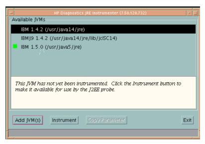
The Instrumenter lists the JVMs that were discovered by the Instrumenter and are available for instrumentation. The JVMs that have already been instrumented are listed with a green square preceding the name of the JVM.
