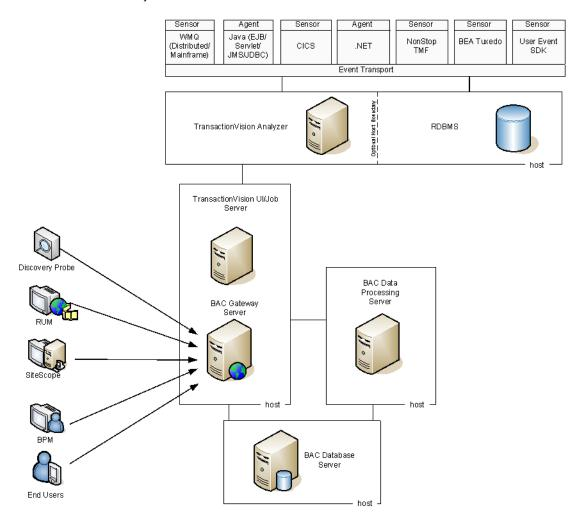
In deployment environments with multiple Business Availability Center Gateway Servers, such as in support of a high-availability scenario, only one TransactionVision UI/Job Server can be running at any given time. You can set up a mirrored UI/Job Server on the other BAC Gateway Server hosts, but it cannot be started until the primary TransactionVision UI/Job Server is stopped.
