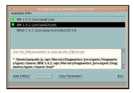
The JRE Instrumenter displays the JVM parameter in the box below the Available JVMs list, which must be used when the application server is started.
