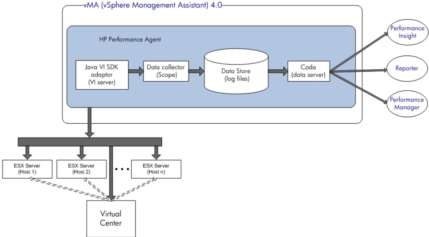
With this solution the HP Performance Agent is installed on a vMA and uses a Java VI SDK provided by VMware to collect performance data from ESX(i) hosts. PA 5.00 includes a Java VI SDK adaptor (VI server) which sources performance data from various ESX(i) hosts, guests and Resource pools. Scopeux, the data collector component of PA spawns the Java VI SDK adaptor which is also known as **VIServer (or VIdaemon )**.
