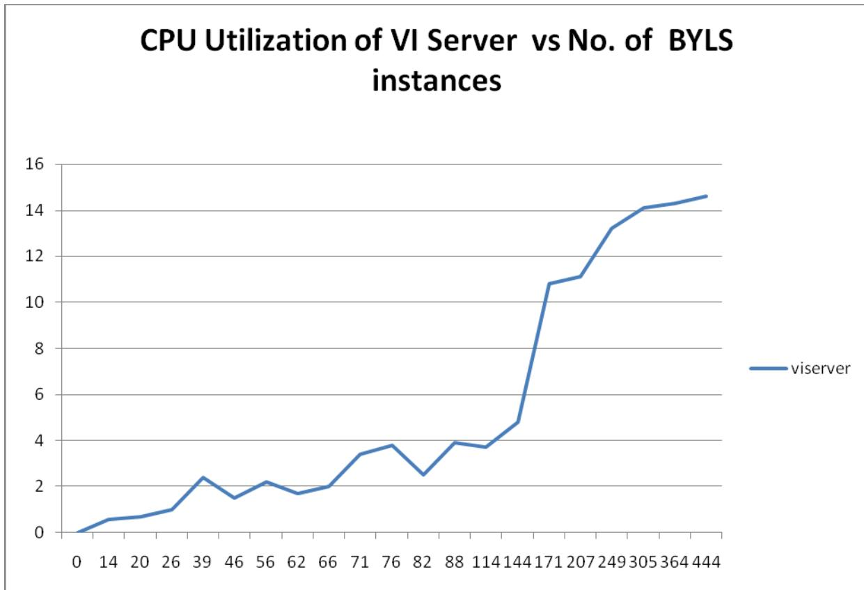
The above graph indicates that after number of BYLS instances crosses 170, there is steady increase in CPU consumption by VI Server during data collection. When number of BYLS instances is below 170, there is varying CPU consumption.
