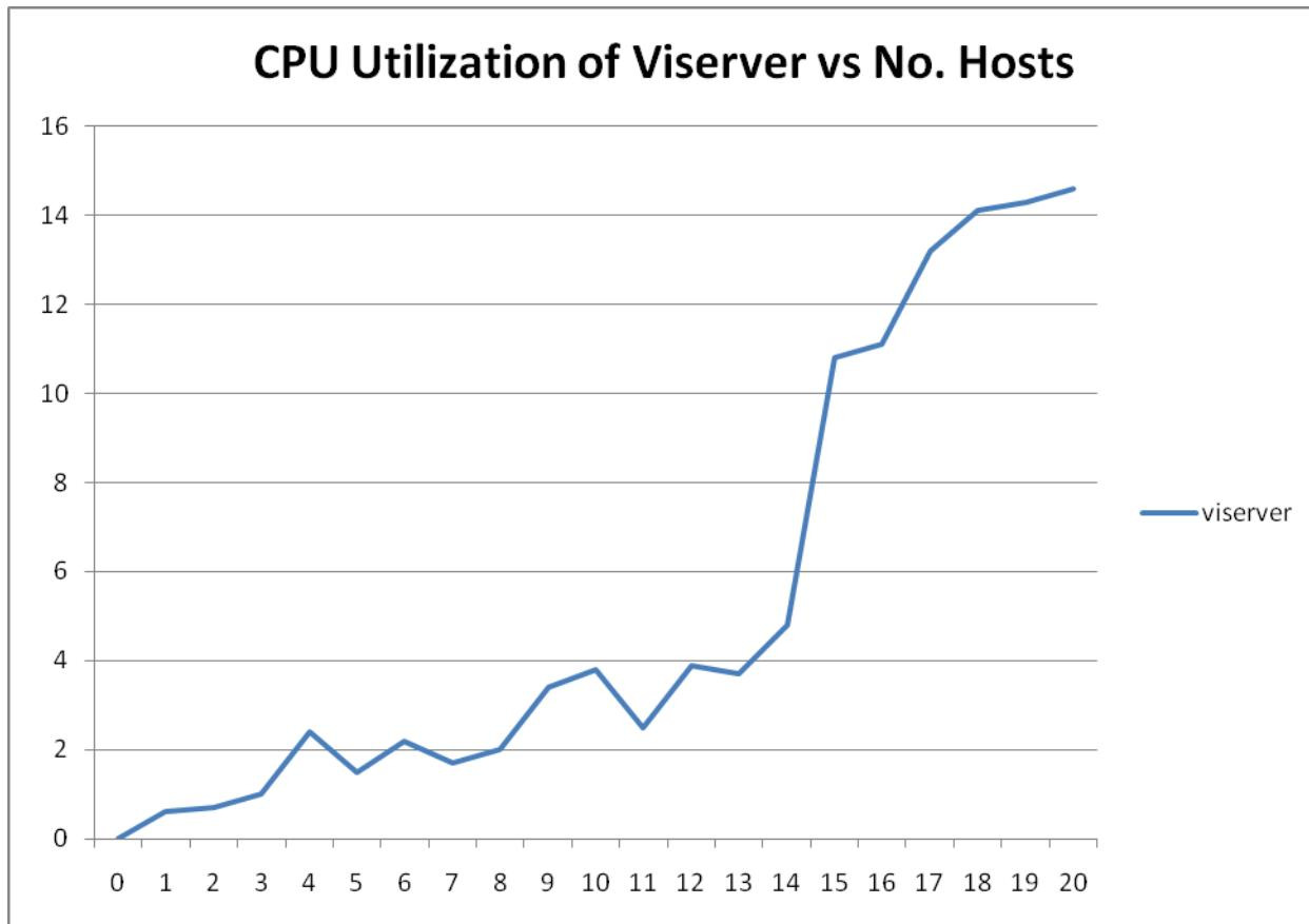
As the number of ESX(i) hosts increases, the CPU utilization of VI Server stays with a range (0-5 %) up to 14 ESX(i) hosts. After number of ESX(i) hosts is increased and is more than 14, CPU utilization gradually increases during data collection with every host added. Note that this CPU utilization peaks at end of the sampling interval ( which is 1 minute or 5 minutes).
