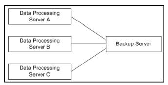
For example, in the above diagram, when Data Processing Server A fails, its services automatically move to Backup Server. When it returns online, it acts as a backup for its original services which are now running on Backup Server. However, Data Processing Server A is not defined as a backup for Backup Server.
