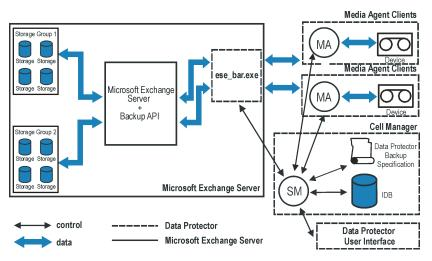
Figure 28 Data Protector Exchange Server integration architecture Table 16 Legend
