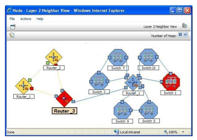
The Status of the Node Down device for a non-SNMP node changes to **Critical** and the device's map icon color changes to red. The Status of the interface on each end of the connection also changes to **Critical** and each interface's map icon color changes to red.
