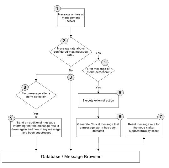
In case of the policy-based message storm (see Figure A), the message rate is reset for policy x on node y after PolicyStormDelayReset.
