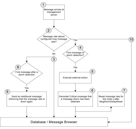
In case of the policy-based message storm (see Figure B), the message rate is reset for policy x on node y after PolicyStormDelayReset.
