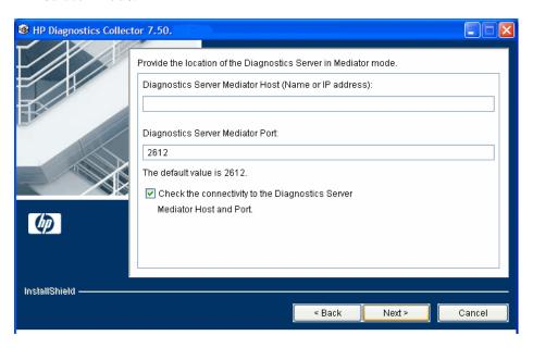
If there is only one Diagnostics Server in the Diagnostics deployment where the Collector will run, enter the host name of the Diagnostics Server and its event port information.
