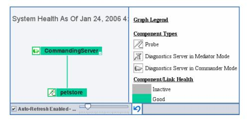
The Java Probe is colored grey in the System Health Monitor when the monitored application is closed. Once the application has been started the Probe is colored green.
