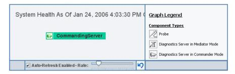
When a Diagnostics Server is deployed in Commander mode, it has both commanding and mediating responsibilities. The Diagnostics Server in Commander mode is represented in the System Health Monitor component map by an icon labelled **Commanding Server**.
