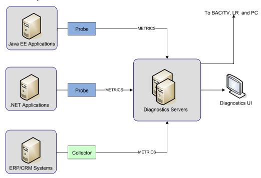
In the diagram displayed above, there is one Diagnostics Server in Commander mode connected to a one or more Diagnostics Servers in Mediator mode. Each Diagnostics Server in Mediator mode is connected to a number of probes or collectors. The Diagnostics probes and the Diagnostics collector capture events from the monitored applications.
