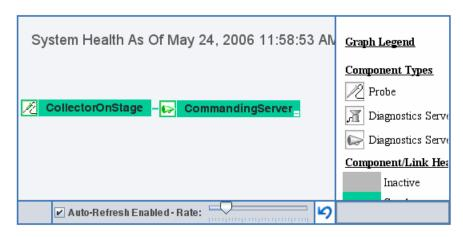
When the Collector has been stopped, the Collector node in the System Health monitor is grey. When the Collector has been started the node is green.
