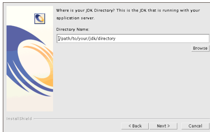
Figure 4.16. Custom installation folder in UNIX - JDK folder used by the application server
