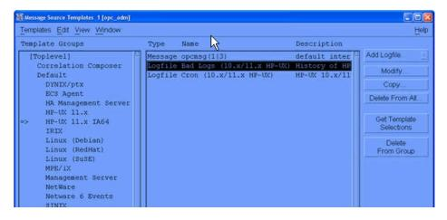
The right pane contains the members of the selected group. For the HP-UX 11.x IA64 group, there is a **Logfile: Bad Logs** item. When this item is selected, it activates the **Conditions** button. Press this button to edit the configuration of the Logfile Bad Logs template. This displays the Message & Suppress Conditions window.
