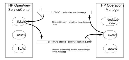
This mode is constructed through the registered connection from OMU to ServiceCenter via the MSI API, as well as the MEI API. This mode will invoke the following components of SCAuto for OMU:
