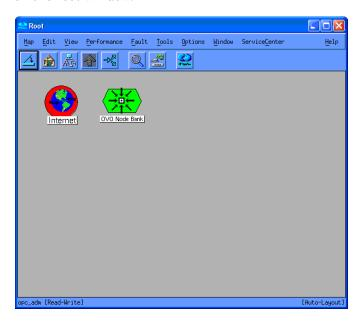
In addition to the root window, the OMU Node Bank window has a similar menu and icon to launch a connection to ServiceCenter to display specific ServiceCenter windows. In the node bank, it is possible to select a node and connect to the ServiceCenter web tier to view ServiceCenter data on the selected node. For example, this menu item lists incidents on the node.
