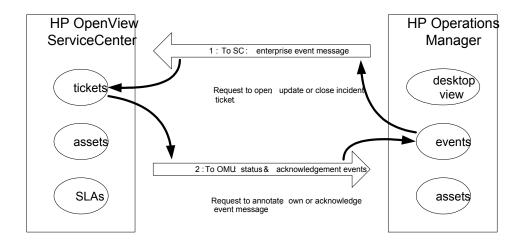
This mode is configured through the registered connection from OMU to ServiceCenter via the MSI API. This mode will invoke the following components of SCAuto for OMU:
