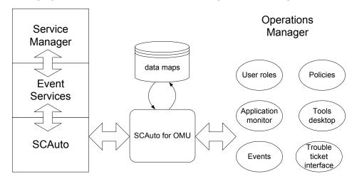
The following figure shows the modular components of SCAuto for OMU in a functional block diagram.
