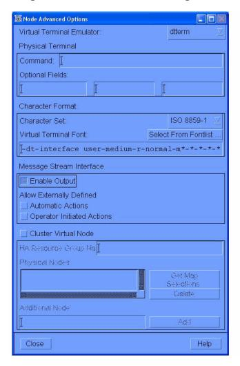
There is one more parameter that must be verified before the configuration is complete. To allow specific nodes to use the MSI or not, OMU has a parameter related to enabling outputs from nodes to the MSI.
