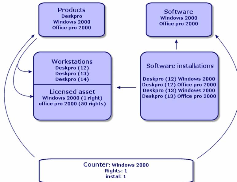
**Figure 4.2. Simplified diagram of software management (4.0)**
