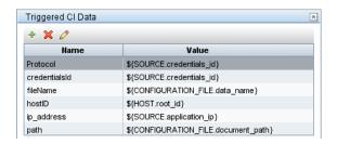
The Trigger CI data is uploaded to the Probe with all variables replaced by actual values. The pattern script includes a command to use the DDM Framework to retrieve the actual values of the defined variables:
