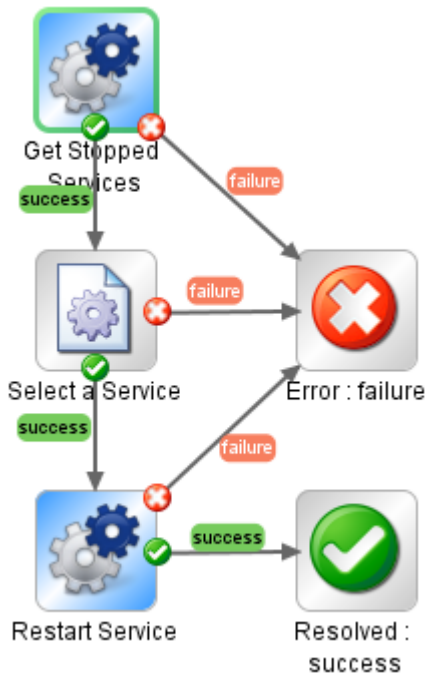
Figure 44 - Transitions in a flow
