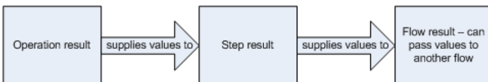
Figure 5 - How an operation's result can become the flow result
