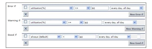
CPU utilization of less than 60% results in a good status; CPU utilization equal to or greater than 60% but lower than 90% results in a warning status; CPU utilization equal to or greater than 90% results in an error status.
