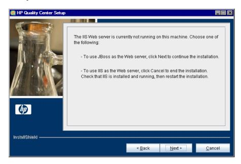
The Quality Center installation can integrate JBoss with the IIS Web server or with the JBoss Web server. Alternatively, you can manually integrate JBoss with the Apache Web server. For more information, see Chapter 6, "Manually Integrating JBoss with Apache." By default, Quality Center integrates JBoss with the IIS Web server.
