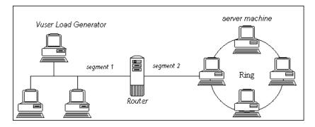
To measure network performance, the Network monitor sends packets of data across the network. When a packet returns, the monitor calculates the time it takes for the packet to go to the requested node and return. This time is the delay which appears in the Network Delay Time graph.
