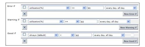
CPU utilization of less than 60% results in a good status; CPU utilization equal to or greater than 60% but lower than 90% results in a warning status; CPU utilization equal to or greater than 90% results in an error status.
