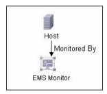
The Host CI has a monitored by relationship with the EMS Monitor CI. The EMS Monitor CI passes status onto the Host CI.
