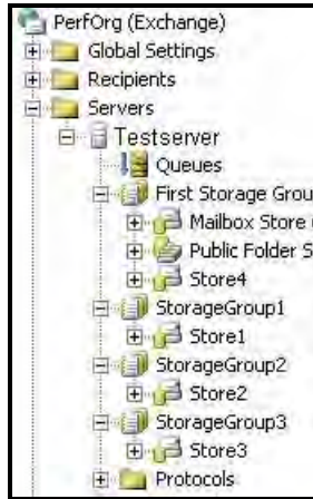
Figure 15. Exchange System Manager with additional storage groups and additional mailbox stores
