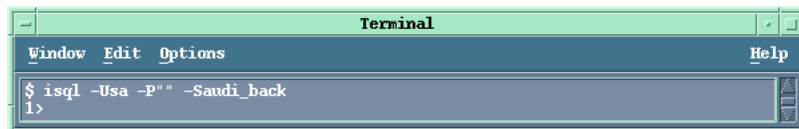
Figure 1-54 Checking if Sybase Backup Server Is Running on UNIX Systems
