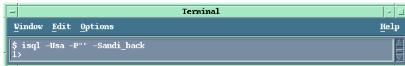
Figure 1-60 Checking if Sybase Backup Server Is Running
