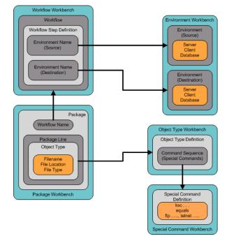
Figure 2-3. How a package comes together
