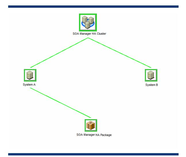
When a system failure occurs on System A, the cluster initiates switchover of the Resource Group from System A. The Resource Group is stopped on System A and started on System B as shown in the following figure.
