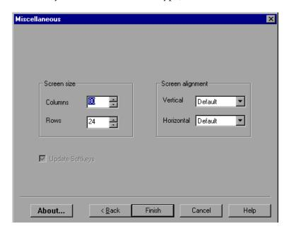
**Note:** The screen size for some emulators is constant (24X80) and cannot be changed during installation. The size of the screen for these emulators is changed by opening the *wrun.ini* file and changing the value of the columns and rows manually.
