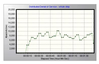
**Note:** To obtain data for this graph, you need to execute one of the following canned security scripts: SYN FLOOD DDOS Attack or UDP Echo DDOS Attack.
