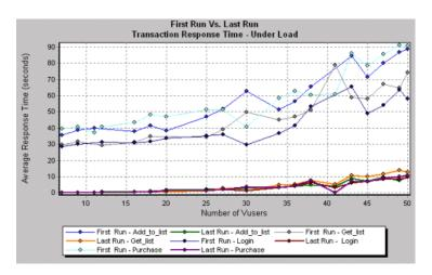
The first load test demonstrates the application's performance in its initial state, before any load testing was performed. From the graph, you can see that with approximately 50 Vusers, response time was almost 90 seconds, indicating that the application suffered from severe performance problems.
