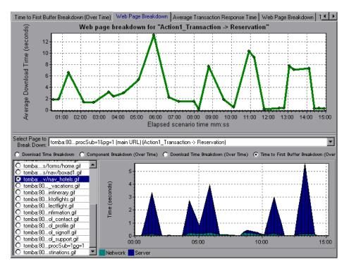
The above graph demonstrates that the server time was much higher than the network time. If the server time is unusually high, use the appropriate server graph to identify the problematic server measurements and isolate the cause of server degradation. If the network time is unusually high, use the Network Monitor graphs to determine what network problems caused the performance bottleneck.
