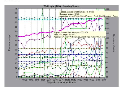
The above graph, therefore, indicates that these two measurements contributed to the slow performance of the WebLogic (JMX) application server, which affected the response time of the SubmitData transaction.
