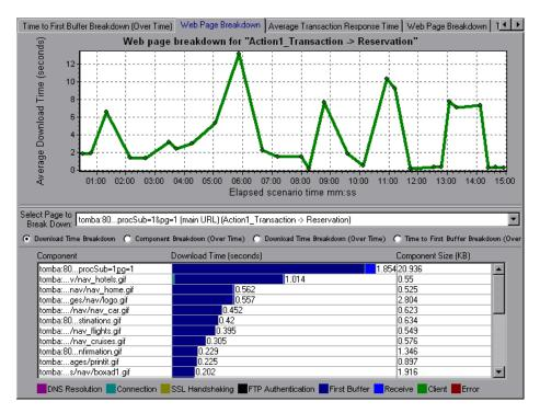
If the download time for a component was unacceptably long, note which measurements—DNS resolution time, connection time, time to first buffer, SSL handshaking time, receive time, and FTP authentication time—were responsible for the lengthy download. To view the point during the scenario at which the problem occurred, select the Page Download Breakdown (Over Time) graph. For more information regarding the measurements displayed, see "Page Download Time Breakdown Graph" on page 233.
