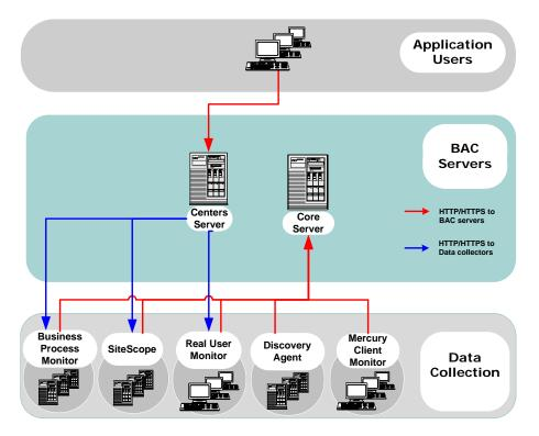
Communication channels between Mercury Business Availability Center servers, data collectors, application users, and Mercury Business Availability Center platform components use various protocols on specific ports. For details, see "Port Management" in *Hardening the Platform*.
