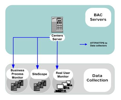
**Note:** In this situation, the Centers Server acts as a client connecting to the data collector using SSL (if required by the data collector).
