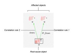
Use the **Show Problem Isolation** option on the IP CI to view, in one step, that the source of the failure is the Network CI.
