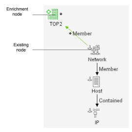
By placing an enrichment node within a TQL context, it receives data from the attributes of the other enrichment nodes in the TQL, and uses it to insert new information into the database that is inferred from an existing one, or represents existing information in a new way.
