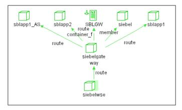
➤ View. Displays all CIs, connected to a selected CI, that are part of the view's TQL, regardless of the layer in which they are located according to the view's folding rules. The View's content is displayed in a new window.
