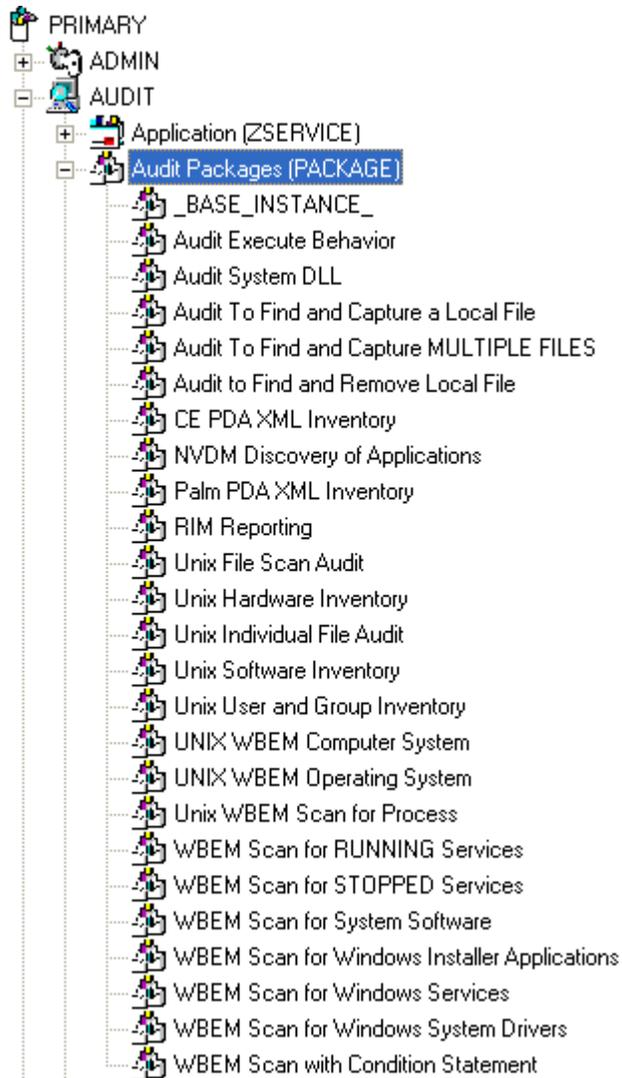
A complete audit service consists of several connected instances in the AUDIT domain. The audit package instance is a container that "owns" the instances connected to it.
