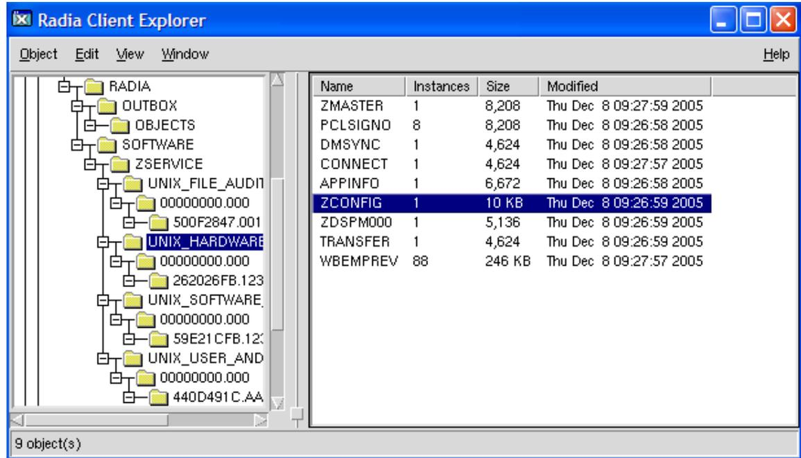
A separate ZCONFIG object is calculated and stored for each service installed or updated during the Client Connect process.
