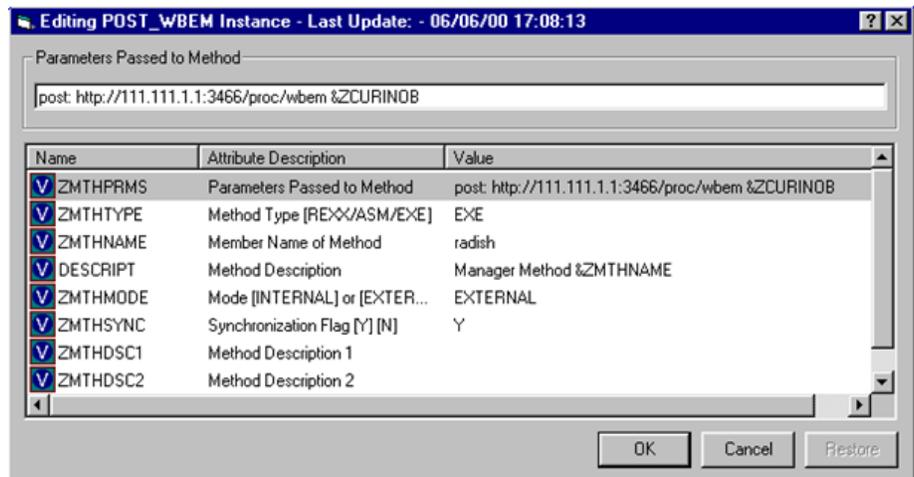
In the example shown, the IP address of the Radia Integration Server has been used. Instead of an IP address, you can use the host name. The port, 3466, is the default port number attended by the Radia Integration Server.
