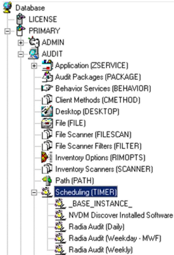
Timers can be set to expire periodically (hourly, daily, weekly, monthly, or at defined intervals), on a specific date, or at a specific time. Each Radia client is installed with the Radia Scheduler service. This service contains an executable timer component that executes any program on the end-user desktop when a timer expires.
