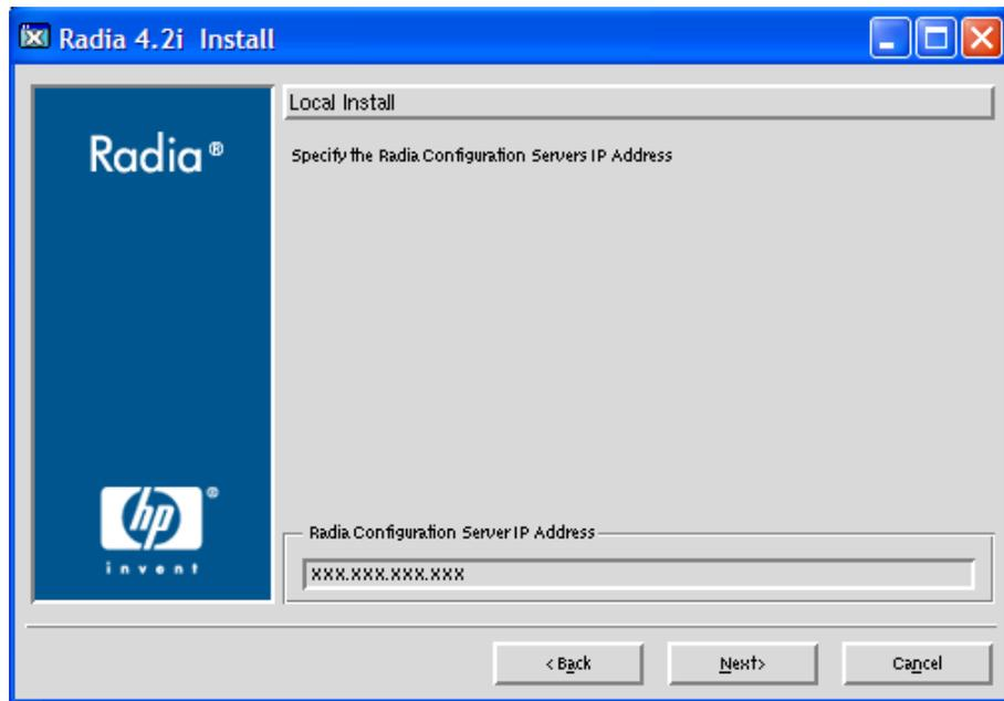
14 Type the IP address (format: xxx.xxx.xxx.xxx) of the Configuration Server to which the Radia client will connect. Specify a valid IP address or hostname recognized by the client workstation.
