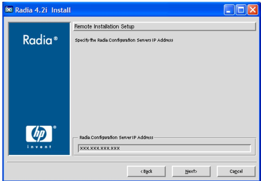
15 Type the IP address (format: xxx.xxx.xxx.xxx) of the Configuration Server that the Radia client will connect to. Specify a valid IP address or hostname recognized by the client workstation.
