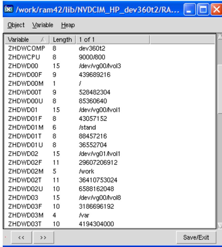
The ZCONFIG object stores hardware information discovered by the Radia client's standard hardware auditing method. Certain types of hardware can occur multiple times. The ZCONFIG object automatically expands to allow additional information to be stored.
