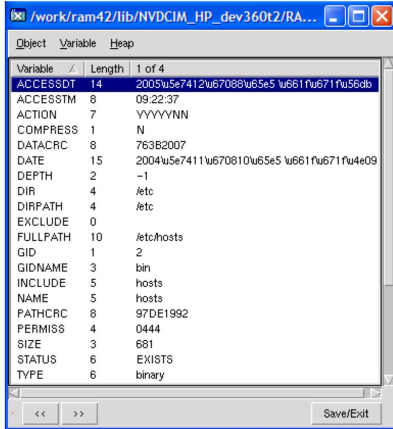
The FILEPREV object contains one heap for each file discovered during the scan for the audit service. It contains the attributes from the AUDIT.FILESCAN class instance that controlled the scan, as described above. It also contains the attributes listed in the table below.
