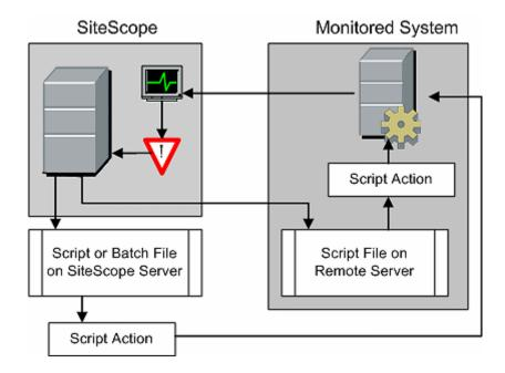
The Script Alert definition or instance and the monitor or monitors that trigger the alert are handled as with other alerts or monitors in SiteScope. For example, you may create a monitor to watch a Web server running on a remote Unix server. You can create a Script Alert associated with that monitor that will execute a script to kill and restart the Web server process if the monitor reports an error.
