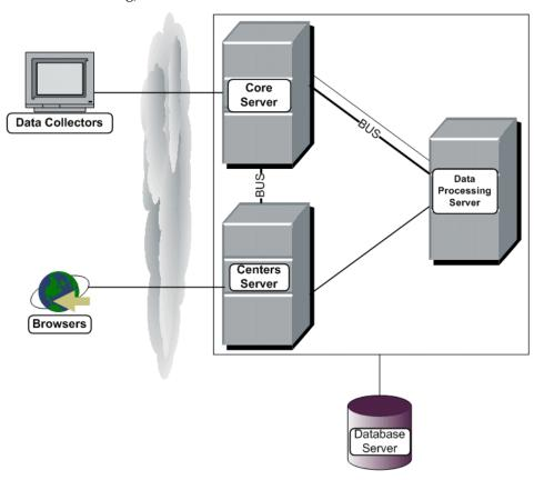
Load balancing (for the Centers and Core servers) and high availability can be implemented in a three machine deployment by adding additional machines. For details on load balancing, see "Load Balancing for Mercury Business Availability Center" on page 40. For details on high availability, see "High Availability for Mercury Business Availability Center" on page 37.
