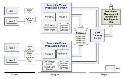
TransactionVision agents collect events and send them via communication links to a designated Analyzer. The Analyzer processes the events and builds them into transactions. The Processing Server is a container for the Analyzer and its supporting components as shown above. The Analyzer and Processing Servers write data to the TransactionVision database and to the BSM components.
