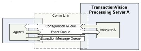
Therefore the host you choose for the Analyzer must be one that supports the message middleware product you want to use to communicate between the agent and the Analyzer. Each type of agent has its own messaging middleware restrictions. See the Deployment Planning spreadsheet (contact HP Software Support for a copy).
