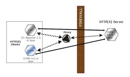
There are different ways to configure HTTP communication in a firewall environment. The recommended way is to use HTTP proxies for OVPA data communication through a firewall. This simplifies the configuration by using proxies that are often already in use in your environment. The firewall must be open for exactly one port if proxies are to be used in both directions.
