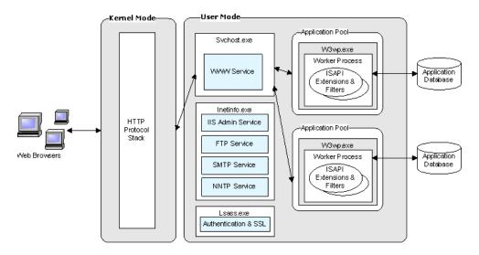
The following diagram illustrates the Worker Process Isolation mode.
