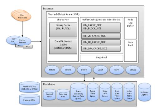
Each Oracle instance uses a **System Global Area (SGA)**, which is a shared memory area, to store its data and control information. The instance allocates itself an SGA when it starts, and deallocates it at shutdown time. The information in the SGA consists of the following elements, each of which has a fixed size, established at instance startup:
