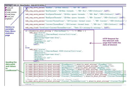
Lastly, as noted above, LoadRunner and Performance Center also allow monitoring of system resource utilization, databases, Web servers, application servers, and so on, using native monitors built into the products or using integration with Sitescope.
