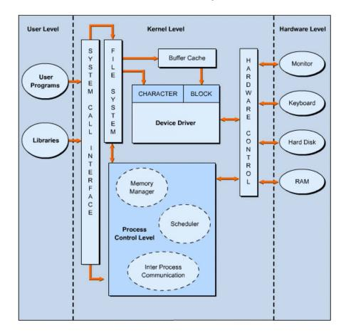
The architecture of the UNIX operating system consists of three levels: **User**, **Kernel**, and **Hardware** as shown on the image below:
