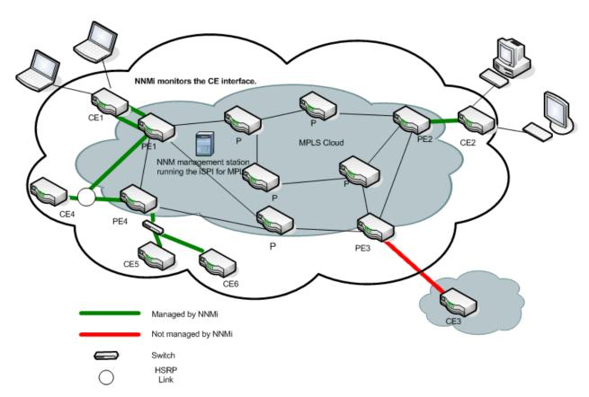
For example, NNMi monitors the CE1 and CE2 nodes and interfaces on the nodes. The NNM iSPI for MPLS helps you monitor the PE-CE communication links. In addition, the NNM iSPI for MPLS helps you monitor two CE interfaces on the CE node communicating with one PE interface and two PE interfaces communicating with one CE interface. The NNM iSPI for MPLS does not monitor the PE3- CE3 link connectivity as the CE3 node is not available in NNMi topology.
