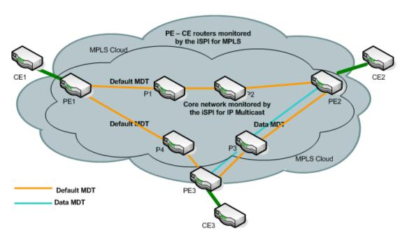
In the example, the NNM iSPI for MPLS monitors the PE routers (PE1, PE2 and PE3) and the PE-CE link (PE1-CE1, PE2-CE2, and PE3-CE3). The core network consists of the PE1, PE2, and PE3 and provider routers (P1, P2, P3, and P4). The iSPI for IP Multicast monitors the traffic flowing from and into the core routers. View the downstream path and upstream path to find multicast flow in the network.
