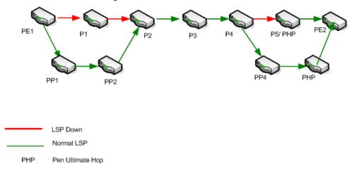
The re-route incident is generated only the first time, in this case the LSP is first Re-routed at PE1 and then again at P4. The re-route incident is generated at PE1.
