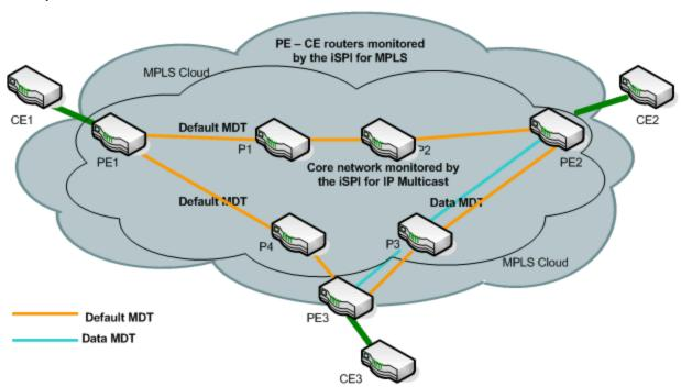
The PE routers (PE1, PE2, and PE3) are monitored by the NNM iSPI for MPLS. The core network consists of the provider routers (P1, P2, P3, and P4). The traffic flowing from or into these core routers are monitored by the NNM iSPI for IP Multicast. You can view the downstream path and upstream path to find the multicast flow in the network. For more information, see <a href="IP Multicast map view">IP Multicast map view</a>.
