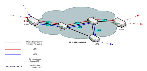
In the example above, there are two LSPs passing through an MPLS cloud. The first one connects the the Edge Routers LER1 and LER3 by passing through P Routers (P1 and P2). The second originates from edge router LER1 and passes through the P Routers P1 and P2, and ends at Edge Router LER2. In this example, LSP1 is mapped to two services and LSP2 is mapped to one service.
