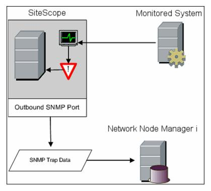
The following diagram illustrates the use of SiteScope as an event data collector for NNMi.
