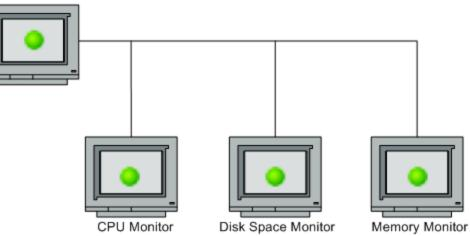
The detailed test monitors can be made dependent on the status of the heartbeat monitor by selecting that monitor. This means the dependent monitors run as long as the dependency condition is satisfied. If the heartbeat monitor detects that the target system has become unavailable, the dependency relationship automatically disables the other monitors. This has the effect of disabling
