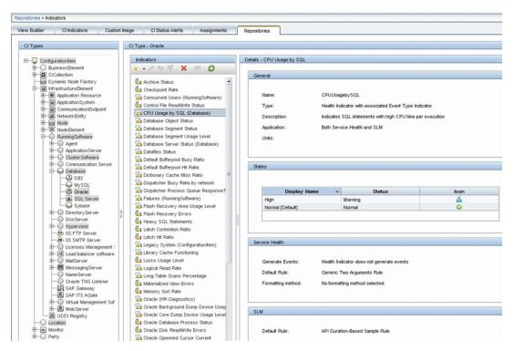
This indicator is defined on the Oracle CI type (the CI that will be reported), and is appropriate for the measurement being read from the log. This measurement describes the amount of CPU that Oracle uses.
