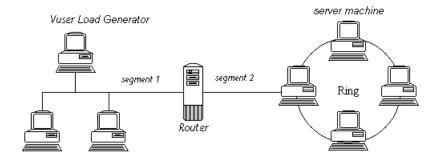
To measure network performance, the Network monitor sends packets of data across the network. When a packet returns, the monitor calculates the time it takes for the packet to go to the requested node and return. This time is the delay which appears in the Network Delay Time graph.
