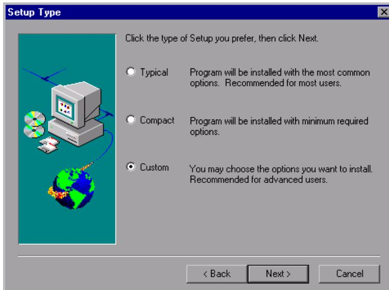
A **Typical** installation installs commonly used program files, including online documentation and samples, the Unified Report, WebTest Add-in , and add-in support for PowerBuilder, Visual Basic, and ActiveX environments. Note that you can choose which add-ins to load at the beginning of each WinRunner session. For additional information on loading add-in support, refer to the *WinRunner User's Guide*.
