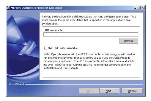
Enter the path to the JVM executable (java.exe) used by the application server that you are monitoring. For example, if you have installed WebLogic 6.1 in your **D:\bea** directory, the **java.exe** file can be found in **D:\bea\jdk131\jre\bin**:
