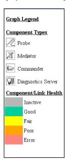
Idle Probes query the Commander for available Mediators on their LAN every 90 seconds by default, and then try a handshake with each of the Mediators. If one or more of the handshakes is not successful, the probe turns red.
