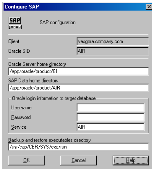
Figure 33 Configuring an SAP R/3 database on a UNIX system (operating system authentication mode)
