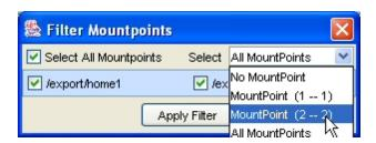
When you are done selecting mount points, click **Apply Filter**. In the following example, all of the mount points are selected. All of the database control files are now displayed, and the database instance sybsystemprocs is shown connected to its logical drive.
