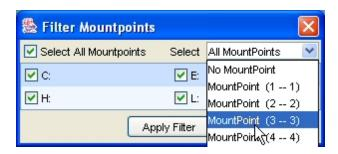
When you are done selecting mount points, click **Apply Filter**. In the following example, all of the mount points are selected. All of the storage groups are now displayed, as well as the connecting switch and storage system.
