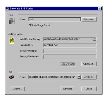
**3** Specify a machine on which VuGen's EJB Detector is installed. Note that the Detector must be running in order to connect. Click **Connect**. The **JNDI properties** section is enabled.
