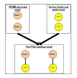
**3** After the federated TQL topology is calculated, the Federation Framework retrieves a layout for the topology result.
