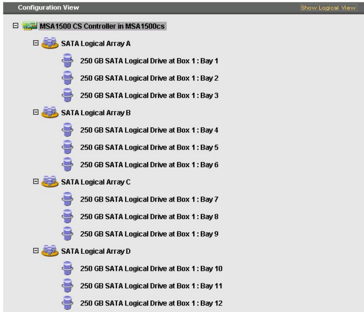
Figure 8. MSA1500 physical array configuration—RAID 0 and four logical arrays
