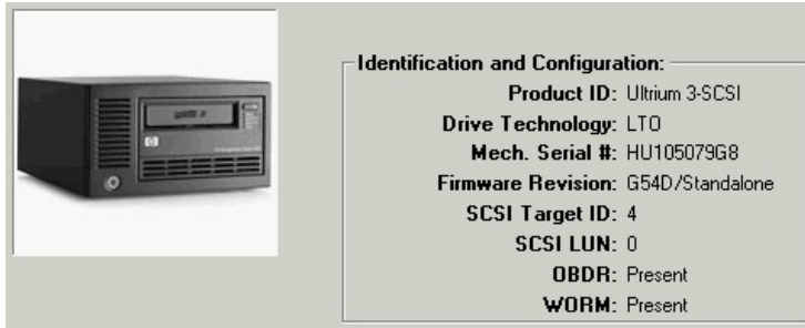
Figure 18. HP StorageWorks Ultrium 960 tape drive configuration
