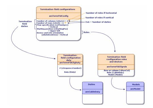
Figure 3.14. Example of termination-field configuration - correspondence at the termination field level
