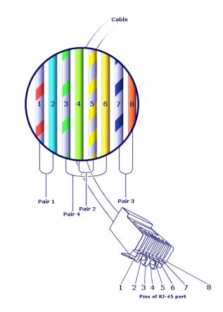
If we take the **RJ-45** connector, each pin is associated with a wire having a given color and a given duty:
