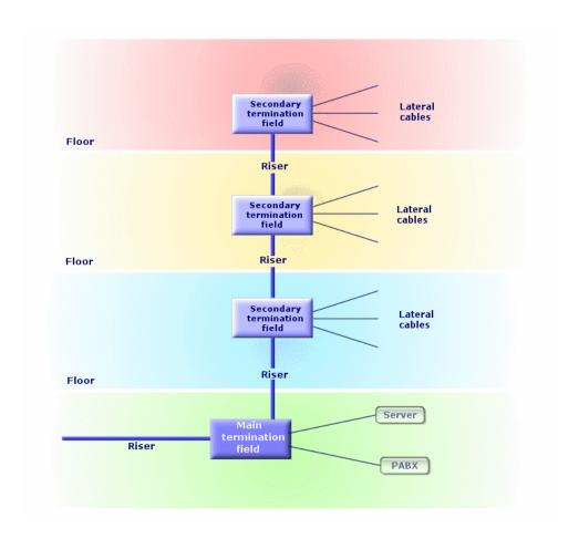
Figure 8.9. Vertical distribution of a cable network - representation
