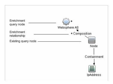
By placing an Enrichment query node within a TQL query context, the query receives data from its attributes, and uses it to insert new information into the CMDB.
