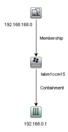
In the example above, the **192.168.168.0** (IP Subnet) CI is linked to the **192.168.0.1** (IP Address) CI through the **labm1ccm15** (Node) CI.
