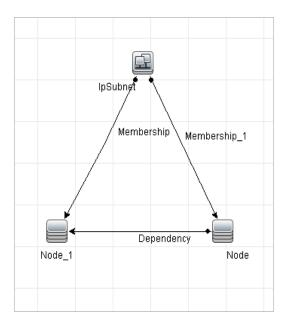
When you consume the view in IT Universe Manager, the relationship between the node CIs (which are under different IP Subnets) is displayed in the higher layer of the view as a relationship between the parent IP Subnets, even though the actual relationship only exists between the CIs in the lower layer of the view. You can double-click the relationship to display the full path between the IP Subnets.
