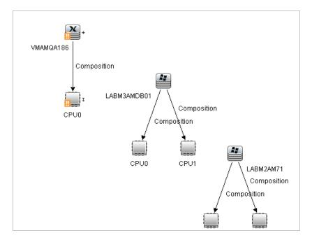
➤ Show Map. A map appears in a separate window containing only the trigger CPU CI and the node CI it impacted. The relationship connecting the two CIs contains the name of the Impact rule defined in Impact Analysis Manager.
